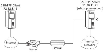
Figure 7.24 The SSH/PPP server architecture.
