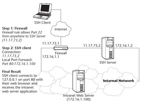
Figure 6.2 SSH local port-forward architecture.
