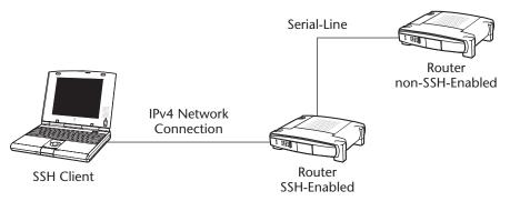
Figure 5.1 Terminal-line access.
